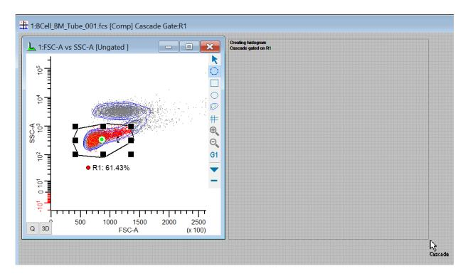
8. Release the mouse button. In the Edit Histogram dialog, select **CD10 PE Cy7** for the X Axis and **CD20 APC** for the Y Axis. Click **OK**. This new histogram will be gated on R1.
